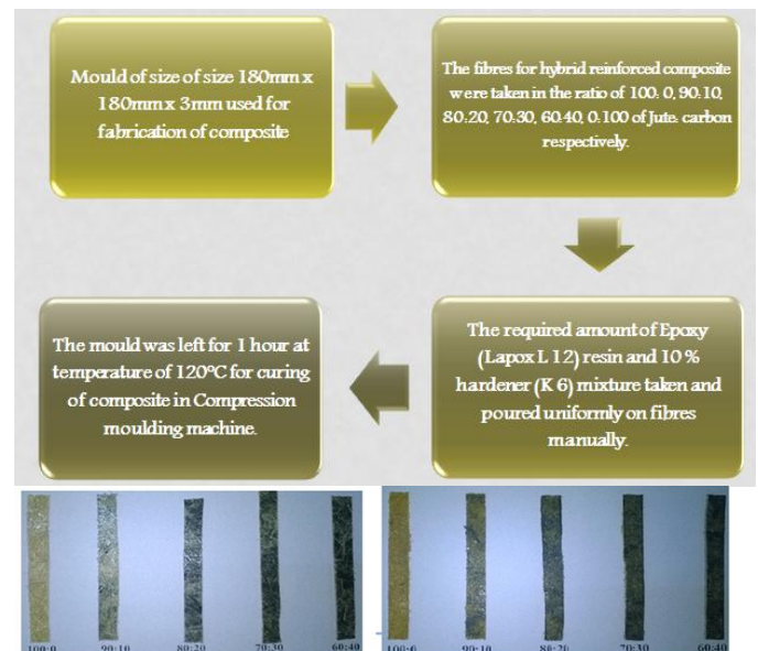
Fig 2 Mould and compound specimen preparation
